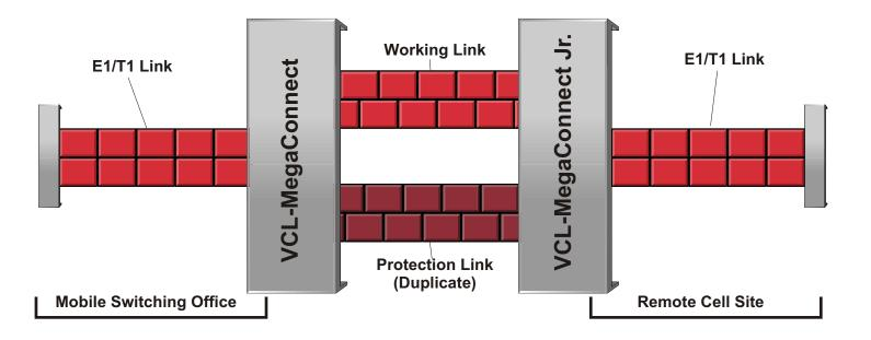
During normal operation, MegaConnect sends duplicate traffic across both the working and dedicated protection E1/T1 facilities while continuously maintaining the performance of both links to determine which link shall be utilized.
