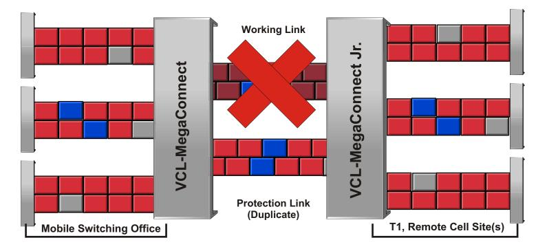
In the event of a failed or degraded T1/E1 link, the traffic is automatically transfered from the previously working link to the duplicate protection link in accordance with the pre-determined operating parameter programmed by the network operator.
