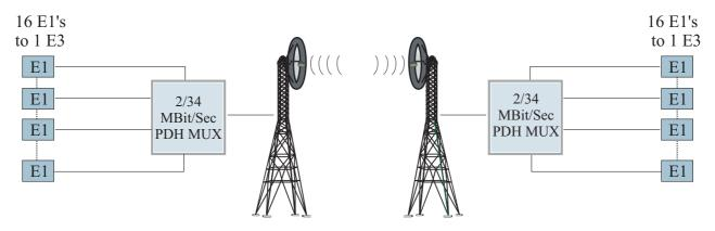
VCL 2/34 Mbps multiplexer with 34 Mbps OLTE (Optical Line Transmission Equipment) 16 E1's 16 E1's to 1 E3 to 1 E3 E1 E1 E1 2/34 E1 2/3434 34 MBit/Sec MBit/Sec MBit/Sec MBit/Sec E1 E1 PDH MUX OLTE OLTE PDH MUX E1 E1
